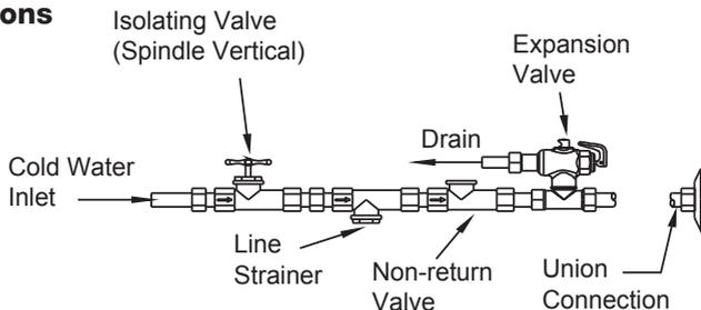
**Note:** a combined isolating valve/non-return valve/line strainer may be used. Expansion valve only required where local regulations demand.
